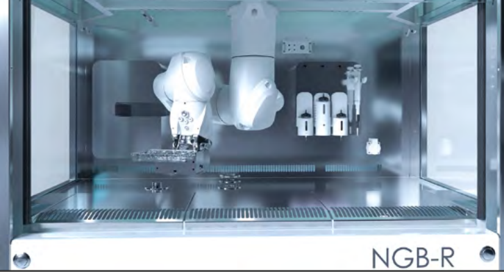
The Poietis NGB platform uses a Stericlean version of the Stäubli TX2-40 robot for 3D printing of human skin tissue.
